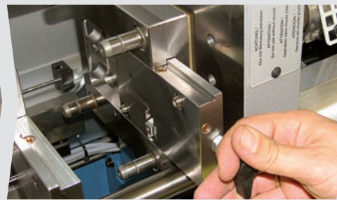
Removable mould inserts for e.g. fast changing / switch
